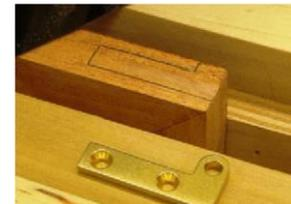
Using a 3/16" bit in a trim router, set the depth of cut to match the hinge thickness. Carefully rout the mortise near the knife lines and finish with a chisel. The finished mortise is shown at the right. Drill pilot holes with a centering bit and fasten the hinge with #4 x 1/2" brass plated screws. Save the hinge's brass screws for final assembly.
