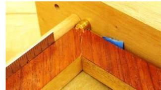
When the door is now slid away, the hinge will remain attached to the base in the precise position required. Disassemble the case and outline the base mortise with a marking knife. Rout the mortise with the trim router and clean it up with chisels. Install the hinge in the base.
