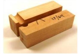
Now check the fit of the pillar and plinth assembly to the case. If the pillar is a bit long, sand the bottom plinth to achieve the fit. Should it be too short, replace the bottom plinth with the 5/16" plinth and sand to fit. If there is a need to increase this thickness a small amount, glue a piece or two of veneer on the bottom plinth's bottom surface. With the fit correct, glue the plinths to the pillars with the chamfers against the beads.
