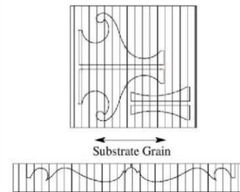
The feet are shown in [Scrolls & Feet](#) drawing. Mill the 1-3/4" wide stock, ripped from *C* when building the case, to 1/2" thickness. Fasten two layers with double-sided tape and attach the foot pattern. Cut and sand to shape. The curved end shape is sanded on a drum sander, fairing the curve with the arc at the end of the bottom scroll.
