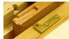
Locating the matching hinge mortises in the base and top presents a precision measurement challenge. The solution is to not do any measurements, but rather just put the door together with the hinges in the correct location.
