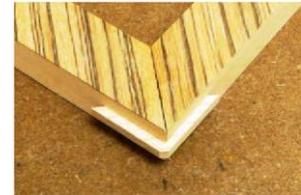
Rip the center door rail 3/4" wide and dovetail it into the side rails. Position the rail so the dial opening in the door is a square. Finally rout the 1/4" x 7/16" rabbets inside the door openings for the glass and clean up the corners with a chisel.
