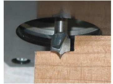
However, the depth of the router cut into the leg needs to decrease to account for the taper. All the dimensions of the reeds decrease in direct proportion to the decrease in the outer leg diameter. So at the 7/8" diameter end, the proportional reduction from the 1-1/4" top diameter is given by the ratio of the diameters.
