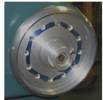
Unplug your lathe for safety and set the index wheel for the first reed. With the router set over the bit relief section at the foot, route the first reed with a slow, firm motion of the router. Do not stop moving the router, or you will end up with burn marks on the reed. Reset the index and repeat until twelve reeds have been cut.
