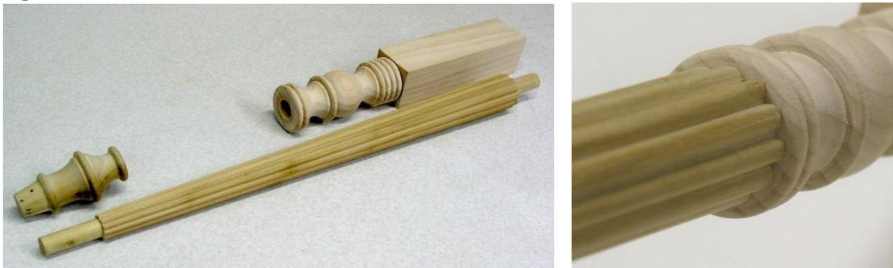
The three parts of the leg are shown above. The top (pilaster end) and foot are conventional turnings with a bored mortise on the mating ends of each. The centered tapered section has turned tenons to mate with the top and foot. Note how cleanly the tapered reeds dive into the surface of the bead. This is a major time saver over hand scraping the reeds and carving the interface.
