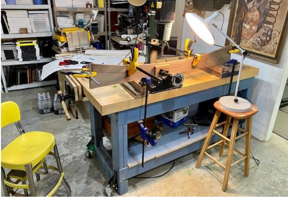
I used the leftover piece of the walnut board I had cut the curved piece from to clamp the curved piece to and “drill” each mortise, moving and adjusting the set-up for each mortise.
