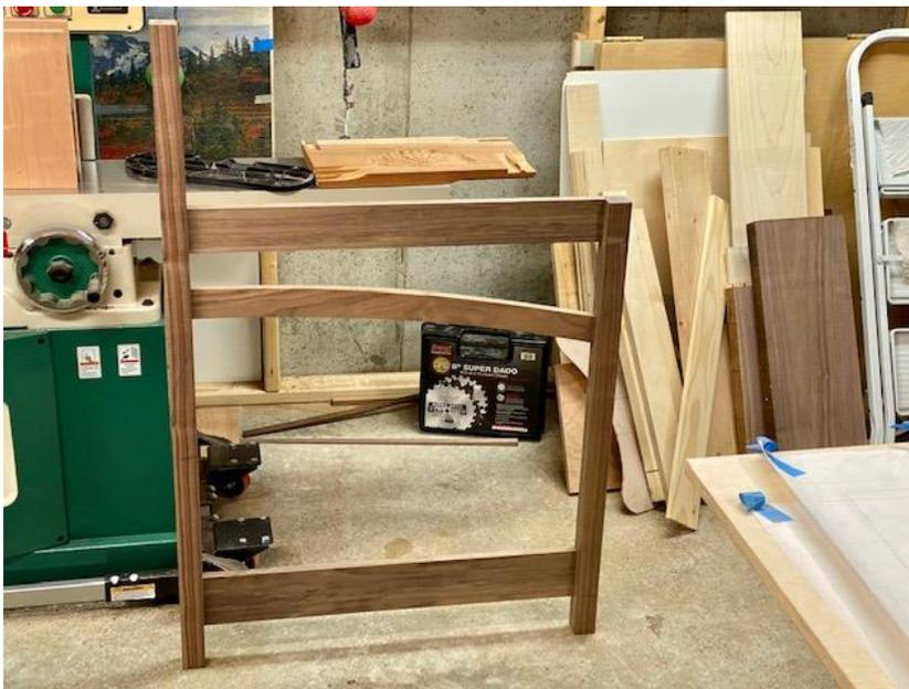
One of the challenges on the project was marking and cutting the mortise and tenons for the curly maple slats on the curved faces. These were marked out using the full scale drawings and made using similar techniques to those described above (see later comments on the footboard).
