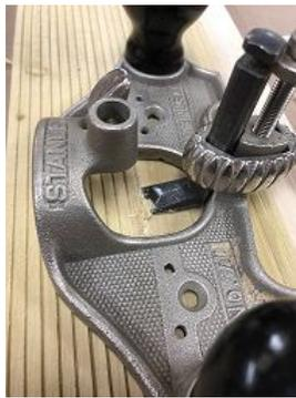
With the clapboards fabricated I transferred the location of each window and door onto the panels. To produce a more realistic look for the doors and windows I flattened those spaces using a router plane. This would also make it easier to attach the window and door frames.
