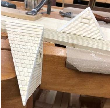
The roof angle was transferred to the gable assembly and a jig was created to hold the gable assembly at the proper angle so that each end could be cut off with the bandsaw. Again the edges were cleaned up with the sander.
