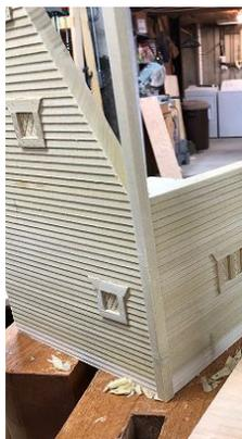
To replicate the corner boards on the house I cut a rabbet into each edge of the end panels. This allowed for a square post to be added. Doing this produced the appearance of corner boards with the proper reveal. The corner posts were glued and pinned in place.
