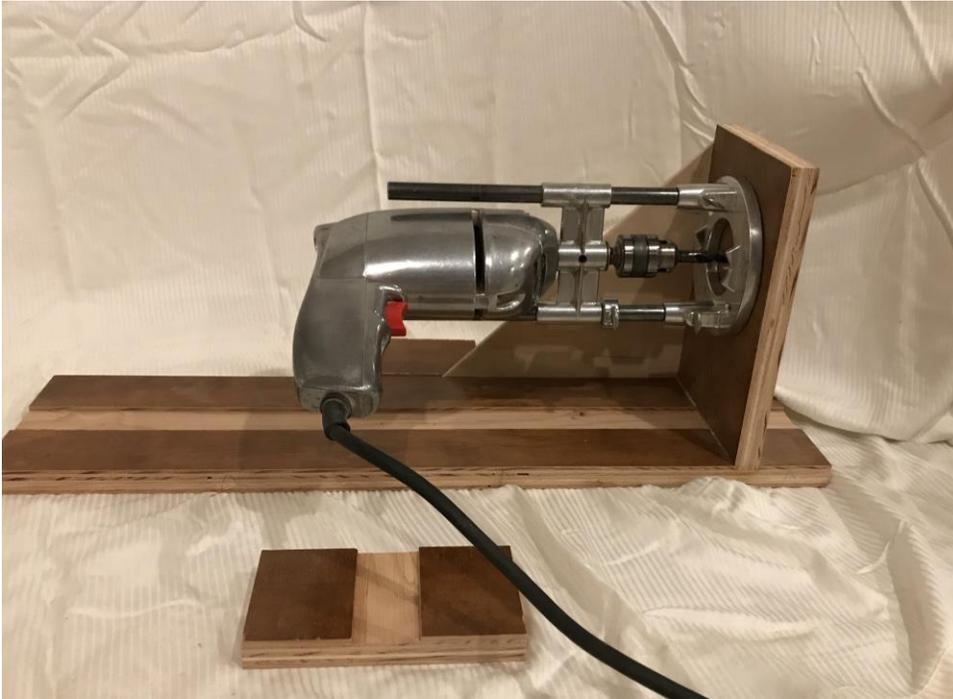
**Figure 5. Jig for Locating Shelf Holes in Legs**
