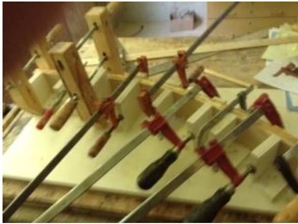
Bending wood is shown with workshop made jig
