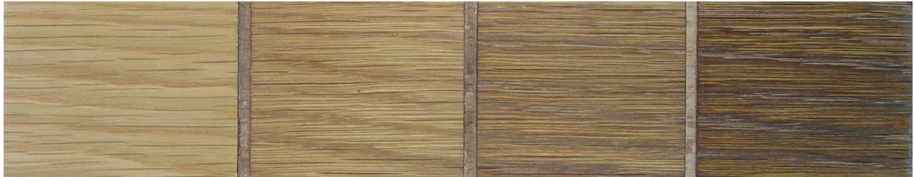
White Oak Stained with 0, 1/16, 1/4. and 1 t/c \text{K}_2\text{Cr}_2\text{O}_7
