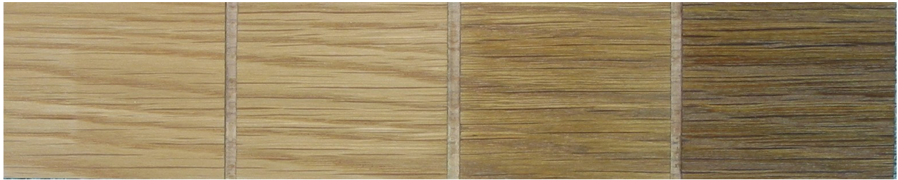
White Oak Stained with 0, 1/16, 1/4 and 1 t/c \text{NaOH}
