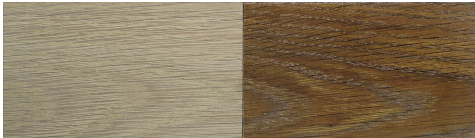
White Oak Fumed for 17 Hours in \text{NH}_3\text{OH}
