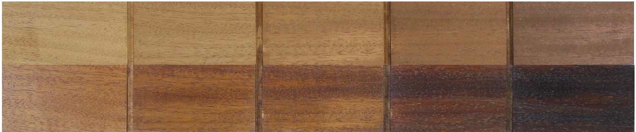
Mahogany Stained with 0, 1/8, 1/4, 1/2 and 1 t/c K_2Cr_2O_7
