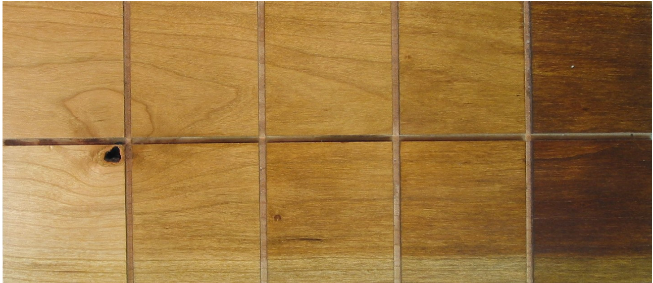
Stained Cherry with Upper Row Exposed to 33 Hours of Sunlight
