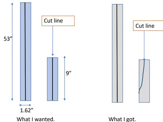
Bottom line: as would be the case for using a table saw, miter saw, jig saw, or even a drill press, setup with a bandsaw is important, and for the resaw operation I would say it is CRUCIAL.
