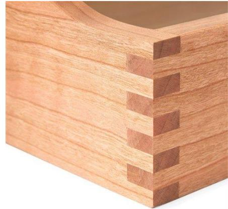
To size the pins and sockets, you simply adjust the width of the dado blade. The blade's height is supposed to match the thickness of the pieces being joined and determines the length of the pins and sockets. Flat-bottomed dadoes are a must for good-looking joints.
